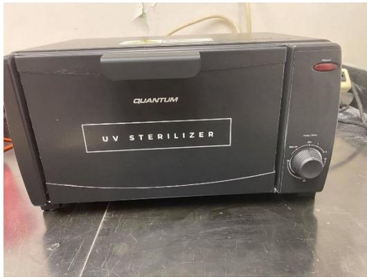
Figure 1. UV machine by Quantum Innovations for disinfection of face masks.
